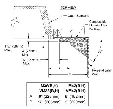
Figure 6 - Side Clearances - Top View (Cross Section)
